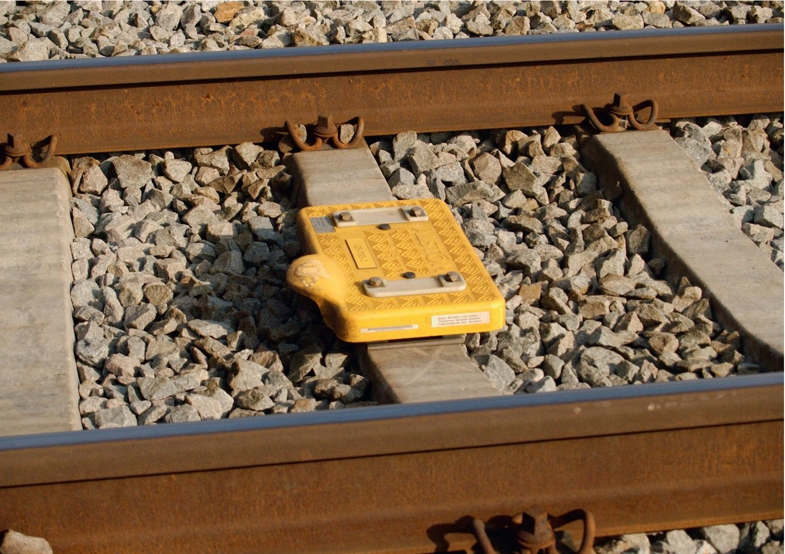
Balise between the rails. ERTMS uses this as a beacon.
