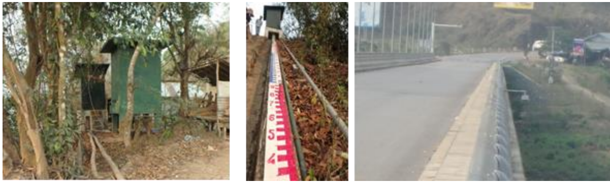
Figure 2: Xayaburi monitoring stations (example): left and middle picture shows new Xayaburi station directly next to existing MRC station, right picture shows radar level sensor on road bridge upstream of Xayaburi dam (Source: MRC, 2018)
