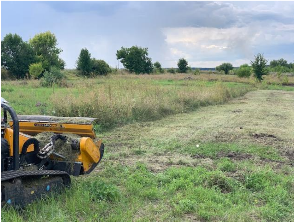
FIGURE 9. THIS REMOTE-CONTROLLED BRUSH CUTTER, USED BY HALO IN UKRAINE, REDUCES VEGETATION CUTTING TIME WHILE ITS OPERATORS CAN REMAIN AT A SAFE DISTANCE.
