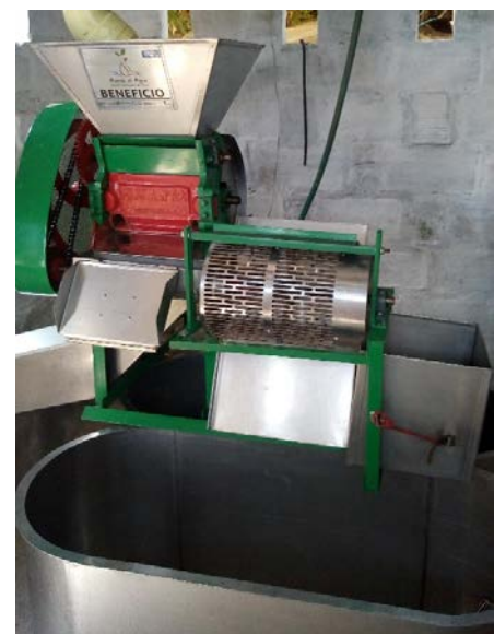
Figure 2: Water-saving coffee-processing equipment installed by GIA project
