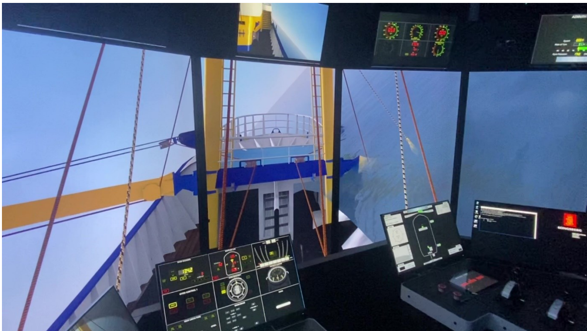
Figure 23: The beam trawler simulator at VDAB during capsizing of the vessel
