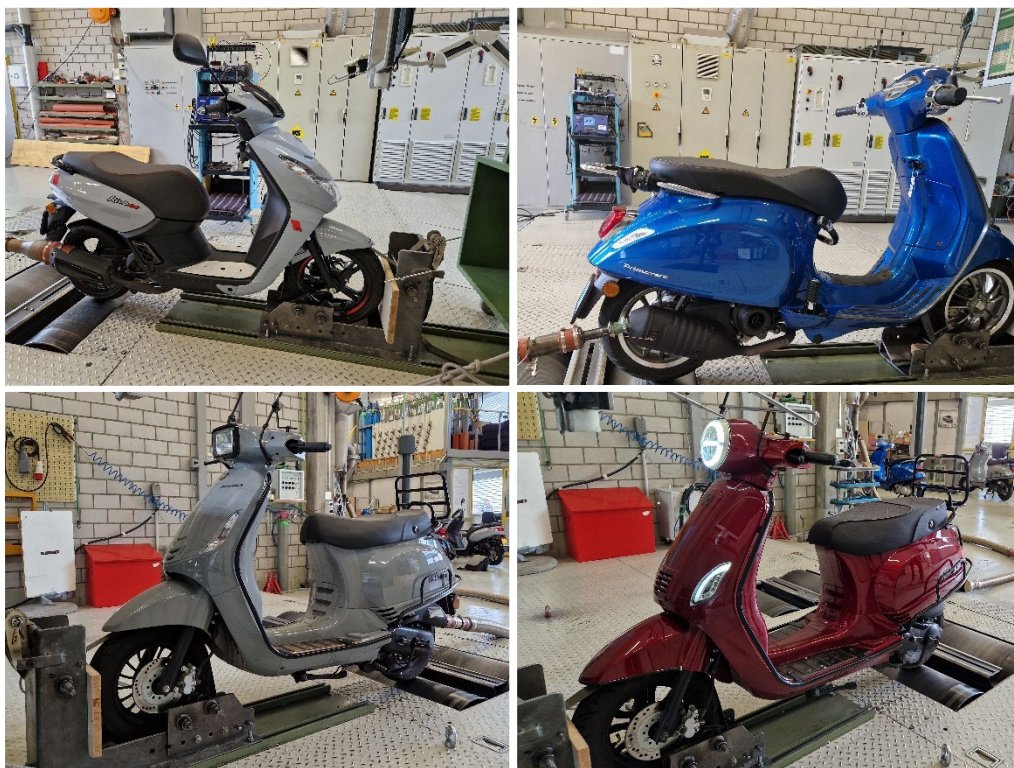
Figure 2: Pictures of the tested Euro 5 mopeds, clockwise: Peugeot Kisbee, Piaggio Vespa Primavera, AGM VX50, La Souris Sourini S
