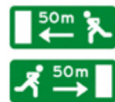
L19 Nearest exit or second nearest exits in the directions and at the distances indicated on the sign
