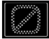
F9 End of all restrictions and advisories indicated on an electronic signaling panel
