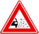
J25 Loose chippings
