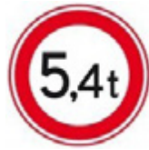
C21 No access for vehicles or combinations of vehicles with a total weight greater than indicated
