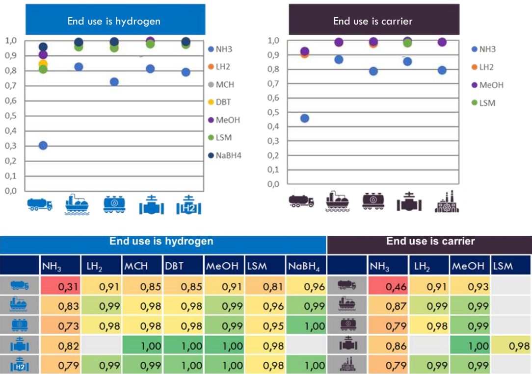
Figure 32: Scores for Safe & Secure for transit and export supply chains in 2030; hydrogen end use and carrier end use
