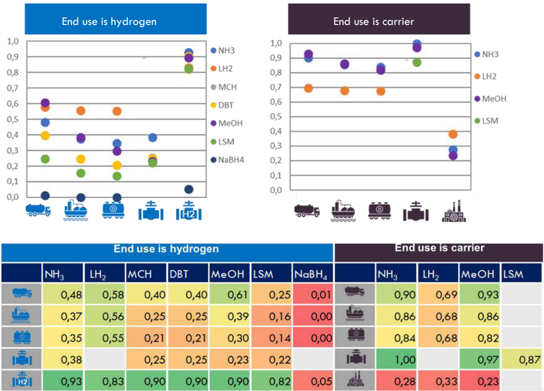
Figure 24: Scores for Economically Robust for transit and export supply chains in 2030; hydrogen end use and carrier end use
