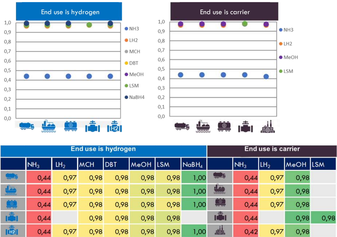
Figure 51: Scores for Fair for inland supply chains in 2050; hydrogen end use and carrier end use
