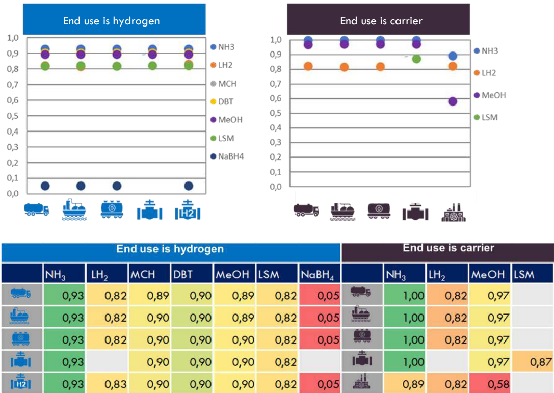
Figure 22: Scores for Economically Robust for inland supply chains in 2030; hydrogen end use and carrier end use
