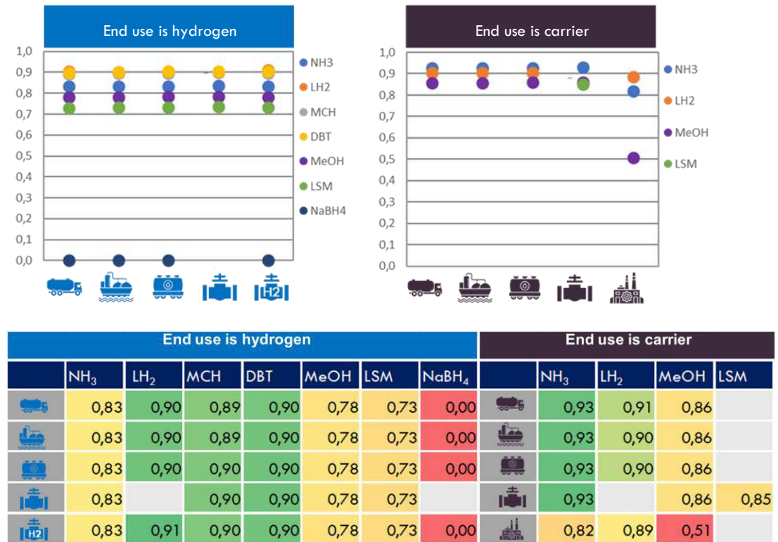
Figure 42: Scores for energy losses for inland supply chains in 2030; hydrogen end use and carrier end use
