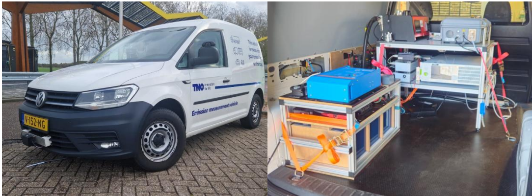
Figure 2.1: TNO plume-chase vehicle: Sample inlets and radar on the front bumper, and the licence plate camera behind the window (left). NO x , PN and CO 2 -measurement instruments and battery pack in the rear cabin (right).
